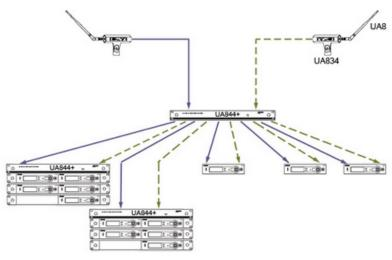
Note: The same configuration is used for 11 to 13 receivers.
