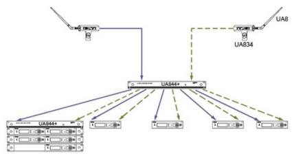
Note: The same configuration is used for 6 to 9 receivers.
