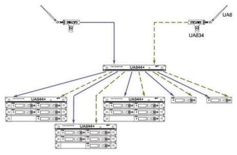
Note: The same configuration is used for 14 to 17 receivers.
